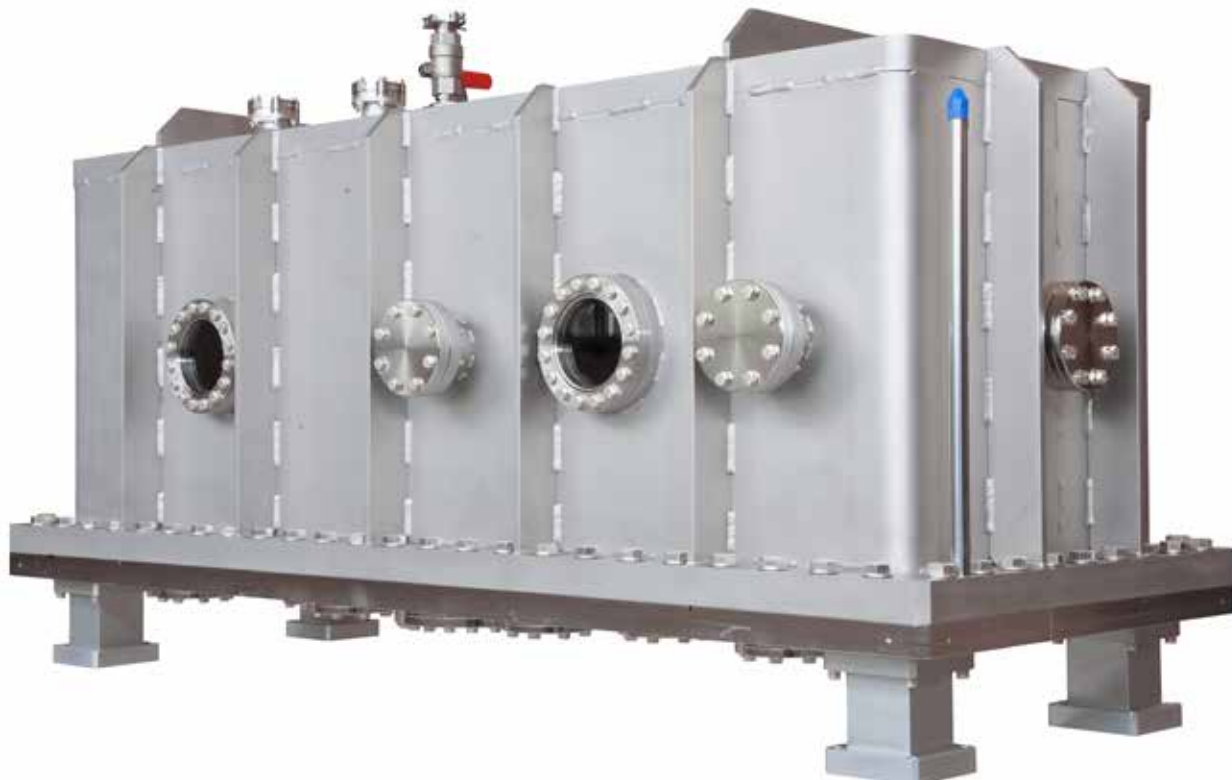
For particle accelerator specialist RI, ALMA produces not only vacuum screws, but also complex chambers.
